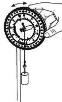
4. Cut a string about 60 cm long. Tie a loop about 25 cm from one end so that the string length on one side of the loop is about 20 cm and the string length on the other side of the loop is 35 cm. Tie one end of the string to the wire hook on one of the Tension Protractors and tie the other end of the string to the wire hook of the other Tension Protractor.
